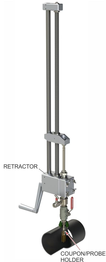
The Sidewinder Retractor comes with a securing nut which attaches to coupon holders, injection tubes and biofilm probes mounted in the standard 1" Access Fitting assembly. Different sized securing nuts and adaptors are available for connecting to electronic probes and alternate sized injection assemblies.
